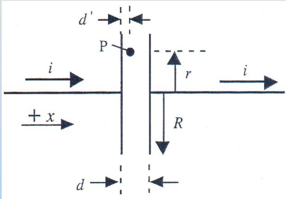
A circular capacitor of spacing  $d$  and radius  $R$  is in a circuit carrying the steady current  $i$  shown.
