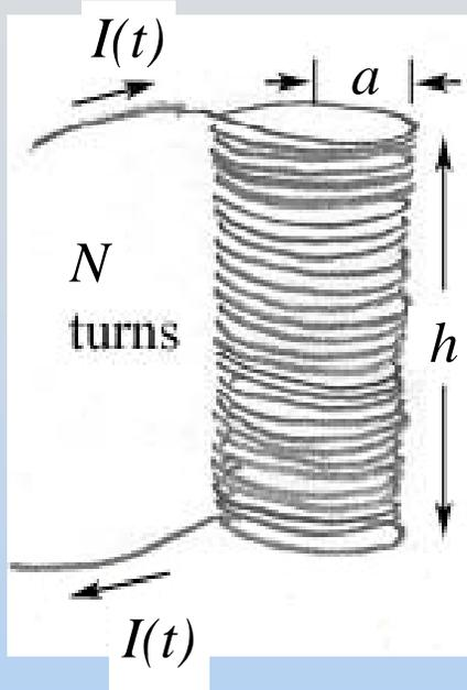
A solenoid of radius  $a$  and length  $h$  has an increasing current  $I(t)$  as pictured.
