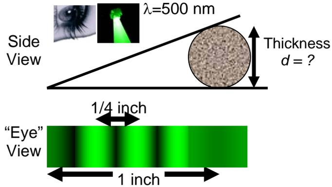
In addition to using hair as a thin object for diffraction, you can also measure its thickness using an interferometer. In fact, you can use this to measure even smaller objects. Its use on a small fiber is pictured at left. The fiber is placed between two glass slides, lifting one at an angle relative to the other. The slides are illuminated with green light from above, and when the set-up is viewed from above, an interference pattern, pictured in the "Eye View", appears.
