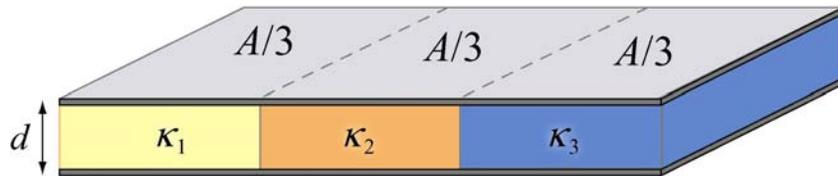
(c) Suppose the capacitor is filled as shown in the figure below. What is its capacitance? Use Gauss's law to find the field in each dielectric, and then calculate  $\Delta V$  across the entire capacitor. Again, check your answer as the dielectric constants approach unity,  $\kappa_i \rightarrow 1$ . Could you have assumed that this system is equivalent to three capacitors in series?
