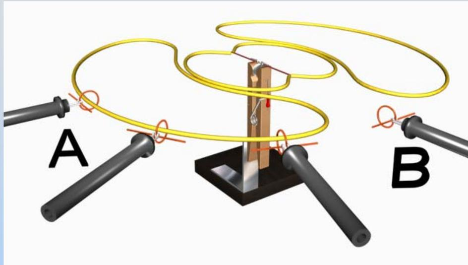
See the E field pattern above. We get maximum power when the line from the transmitter to the receiver is perpendicular to the direction of the antenna (at A). We get (in principle) zero power when the line from the transmitter to the receiver lies along the direction of the antenna (at B).
