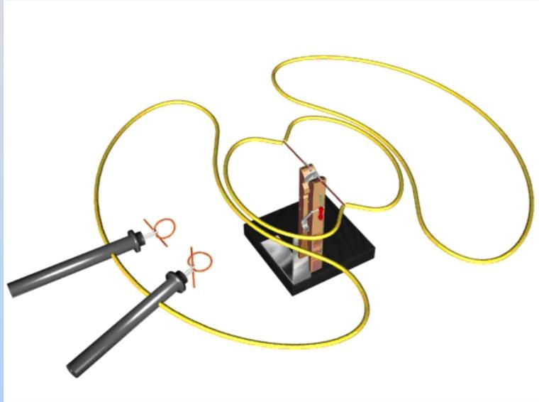
See the E field pattern above. The receiving antenna gets maximum power when parallel to the transmitting antenna wire, because the electric field can then drive the maximum current in the receiver. We say that the wave is “polarized” in the direction of the E field.
