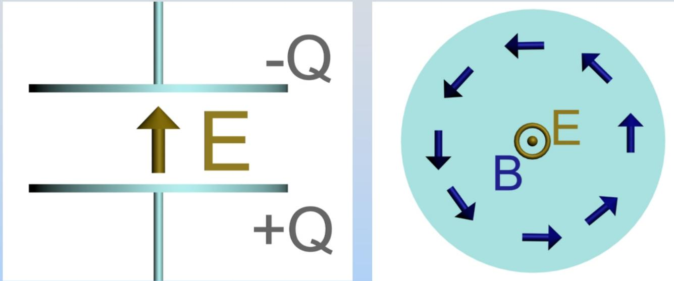
The  $B$  field is counterclockwise, which means that the current (real & displacement) must be flowing out of the page = up. So positive charge is being carried to the bottom plate, and the total charge is increasing.
