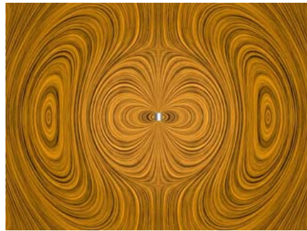
Figure 13.8.6 Radiation from an electric dipole whose dipole moment completely reverses with time ( link )
