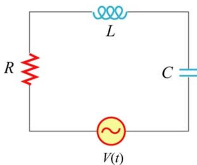
Consider the circuit at left, consisting of an AC function generator ( $V(t) = V_0 \sin(\omega t)$ , with  $V_0 = 5$  V), an inductor  $L = 8.5$  mH, resistor  $R = 5$   $\Omega$ , capacitor  $C = 100$   $\mu$ F and switch  $S$ .
